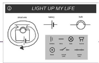
Reviewing the groups' circuit diagrams and the different ways they had drawn the components was a springboard for introducing the scientific symbols for electrical components. We talked about the advantages of having a widely accepted and consistent way of showing electrical circuits. Students then drew over the image to show how they thought electricity flowed in the circuit.
